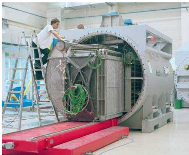
Slika 6: Stacionarna gorivna celica z raztopljenim karbonatom Vir: http://climatetechwiki.org/technology/stationary-fuel-cells
