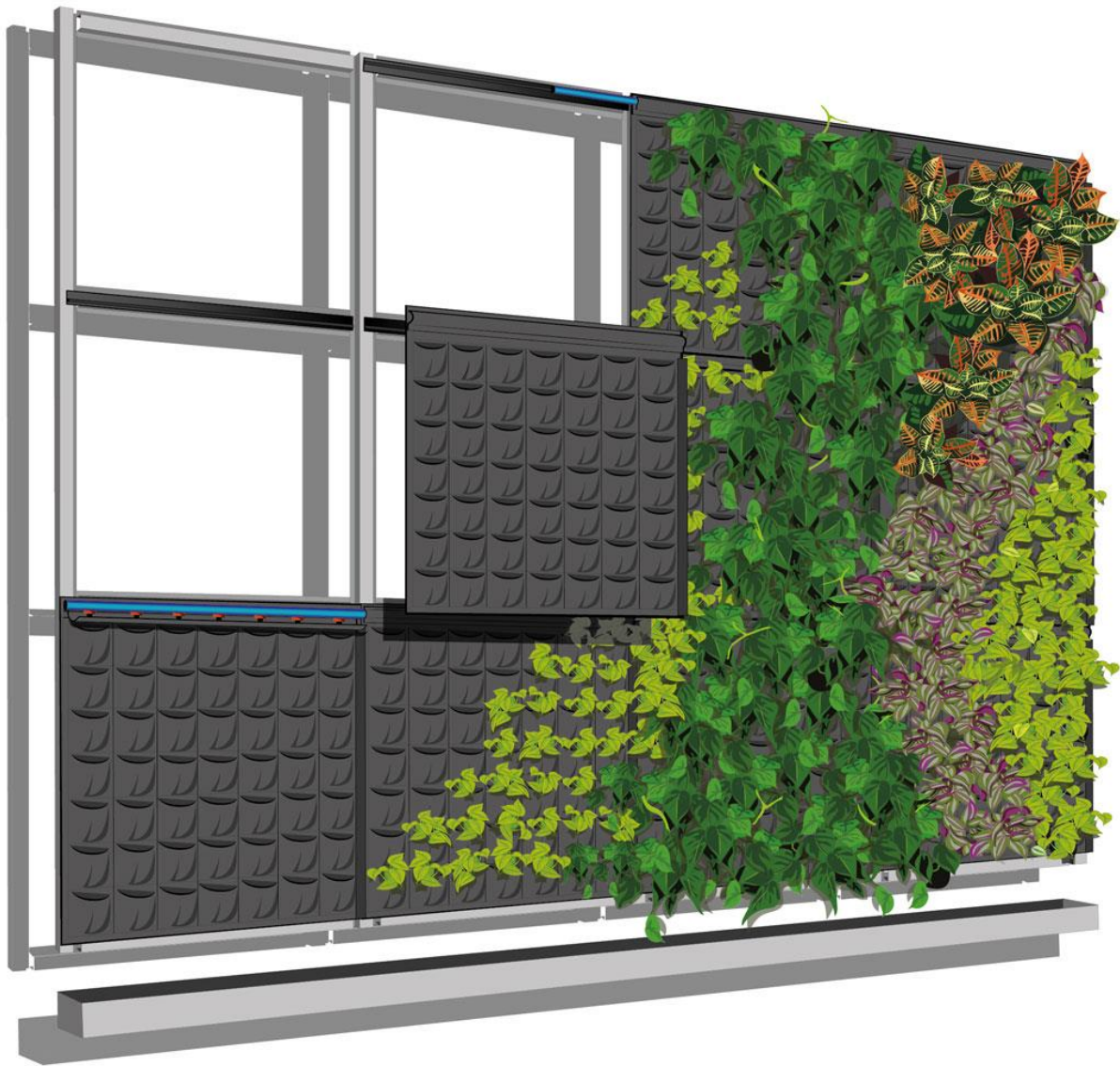
Figure 16: Modular assembly of the Terapia Urbana Fytotextile system
